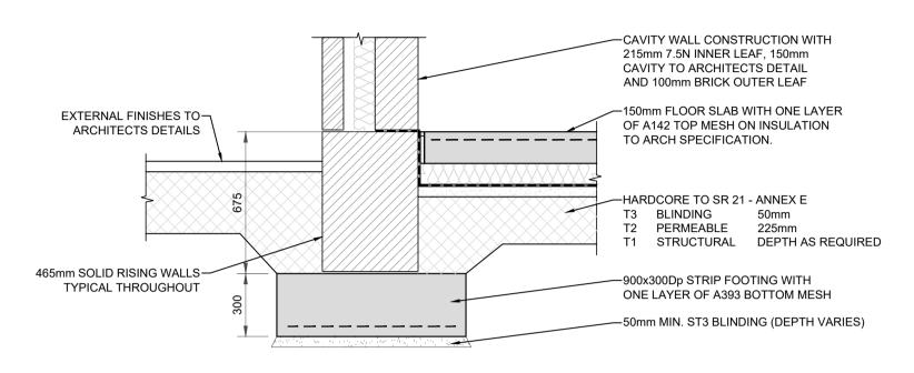
ST2 TYPICAL STRIP FOUNDATION DETAIL Scale: 1:20 100001
