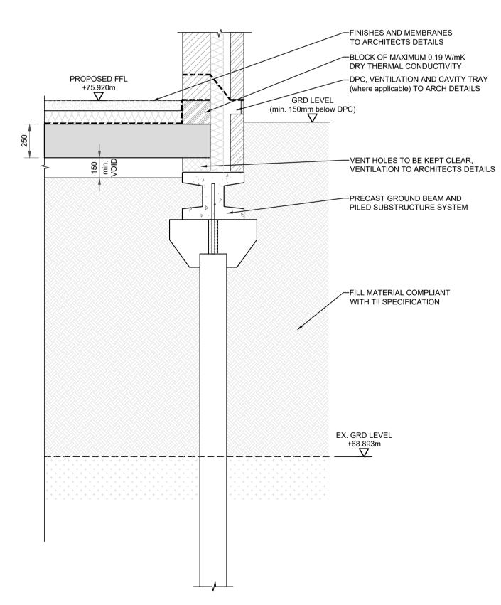
ST3 TYPICAL PILE FOUNDATION DETAIL
